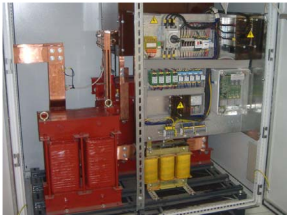
Illustration 9 –Alkaline Electrolyze (400 V AC – 3.300 A DC, 18 V DC, 50 kW 10 m 3 N /h, 32 bar)
