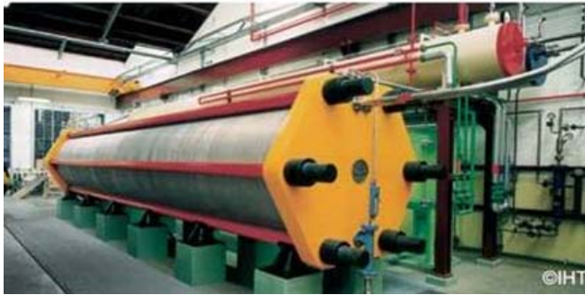
Illustration 8 – Dhejva (Switzerland), Electrolyzer (4 MW, 760 m 3 N/h,) 3rd Meeting Task 24 hosted IHT
