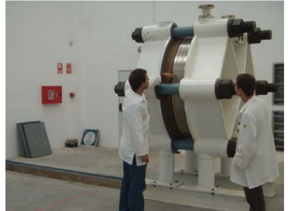
Illustration 9 –Alkaline Electrolyze (400 V AC – 3.300 A DC, 18 V DC, 50 kW 10 m 3 N /h, 32 bar)
